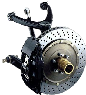
Break system in a car
